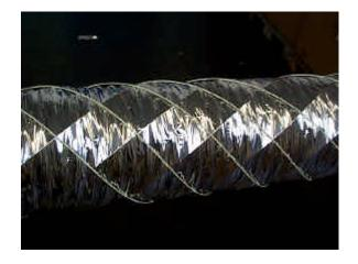
This design is based on reduced conductance through spacers due to several contact points of the spacer strings along the way from the inner to the outer tube.
