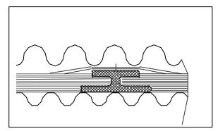
Because of the transferline flexibility there is a need of using more spacing elements than in rigid transferlines.
